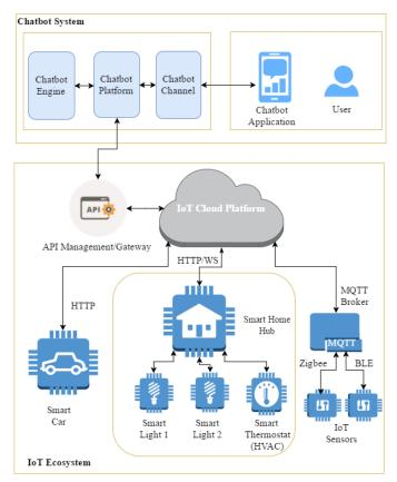
Fig. 3. Proposed System Design of IoT-Chatbot System
